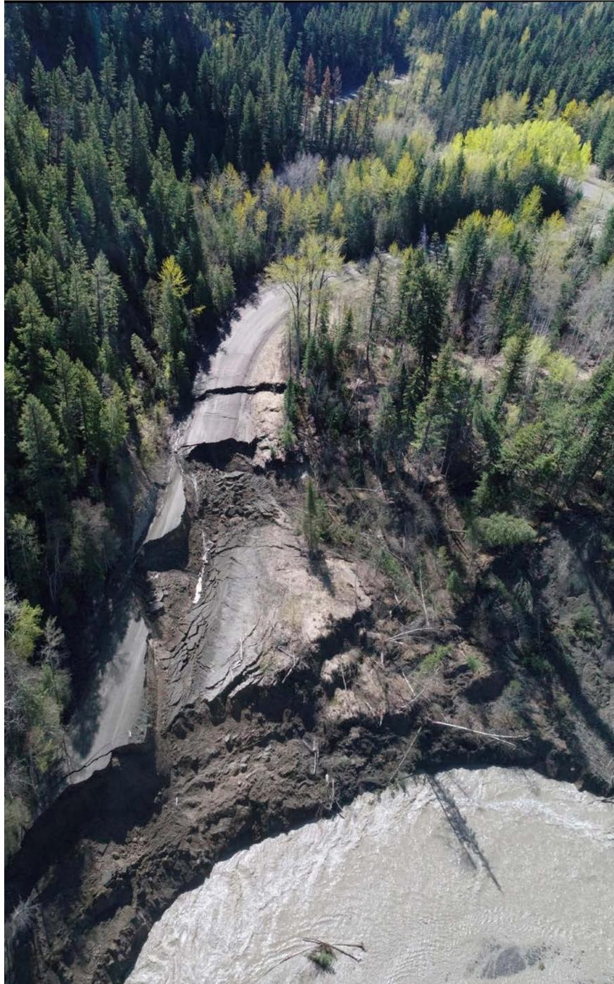
In April 2018, high-water levels from the spring freshet caused Narcosli Creek to erode five sections of the West Fraser Road, on the west side of the Fraser River, approximately 17 kilometres south of Quesnel. Damage was severe, resulting in the road being closed over a three-kilometre section as follows:
