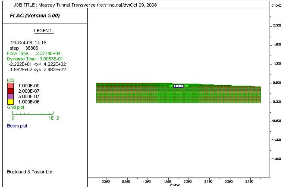
**Figure 1: Model 1 (9% Ground Surface Slope on One Side) Layout and Mesh**
