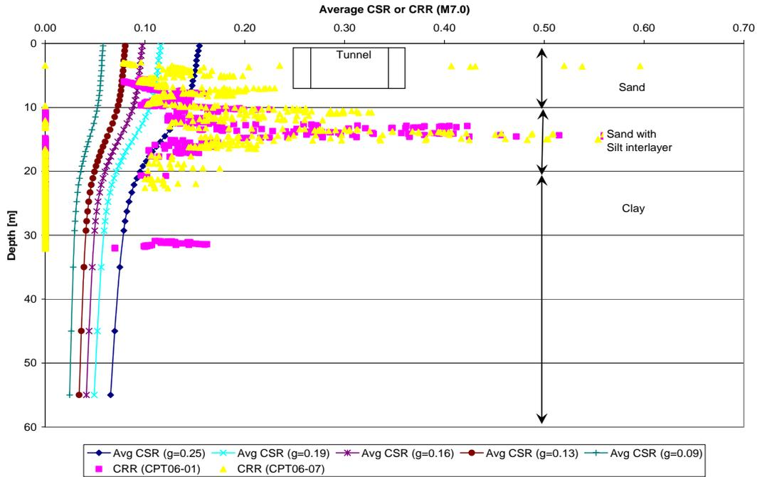
**Figure 5 Average Cyclic Stress Ratios from Scaled Earthquake Motions versus CPT Inferred Cyclic Resistance with Factor of Safety of 1.0**
