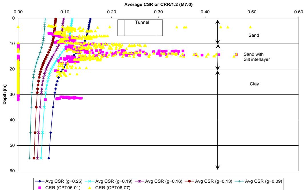
**Figure 6 Average Cyclic Stress Ratios from Scaled Earthquake Motions versus CPT Inferred Cyclic Resistance with Factor of Safety of 1.2**
