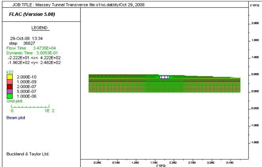
**Figure 2: Model 1 (9% Ground Surface Slope on One Side) with a Continuous Silt Barrier at the Underside of Tunnel**
