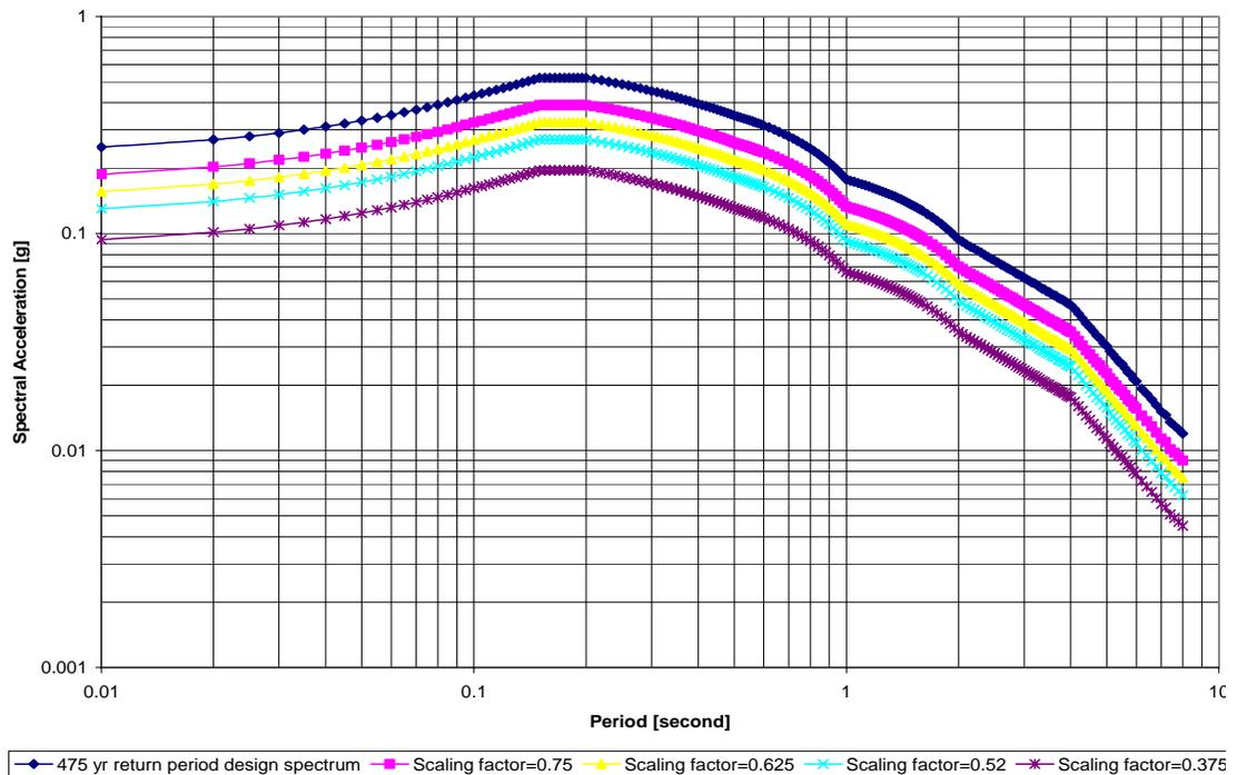
**Figure 4 475 yr Return Period Original Design Spectrum and Spectra for Scaled Earthquake Records Used in This Study**
