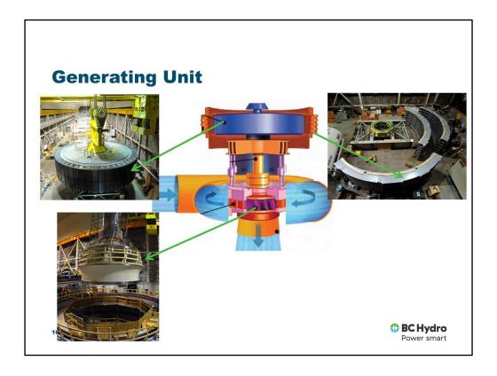
The turbine powers the generating unit that has a moving part—the rotor—and a fixed part—the stator. The rotor's outer surface is covered with magnetized steel plates.
