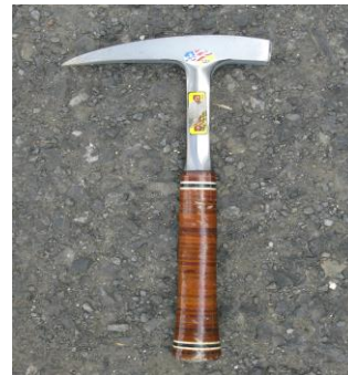
Rock Hammer: one of the oldest prospecting tools
