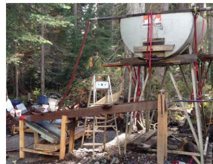
Sluice and water tank used in a small placer mining operation.
