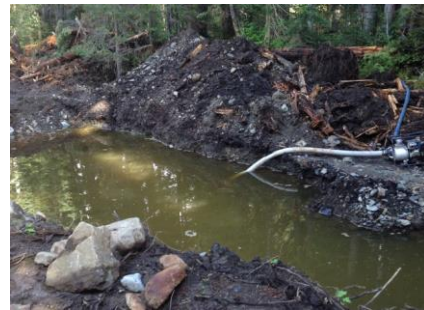
Settling pit used in a small placer mining operation.
